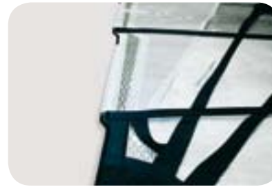
STEP LEECH OUTLINE -creates neutral trailing edge (reduced drag), and promotes smooth progressive twist
