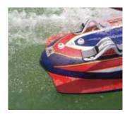
In slightly more wind, the board starts to lift on to its rail, so one wing lifts out of the water while the leeward wing continues to travel below the water surface, acting like an extra fin.
