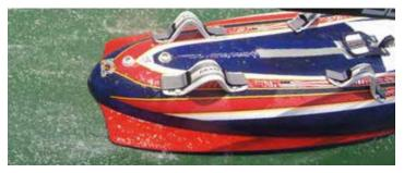
As the board increases speed with in more wind, the wide planing surface starts to generate lift, allowing the board to transition smoothly into planing mode. Because the wings are wide, the planing surface is wide. So the transition into planing is happens earlier than other narrow-tail raceboards.
