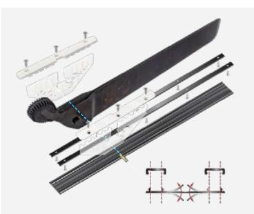
The new tool-free, fully retractable Clipperbox system: the new daggerboard moulds the handle and blade into one piece for a stronger design. The daggerboard can be removed from the board without tools, by positioning the daggerboard at 45 and pulling up. The new rubber lips can be removed and replaced easily also without tools. Featured on the AirPlane, the Inflatable WindSUP Deluxe, the Rio, the Start, the GO Windsurfer and AtomIO Windsurfer.
