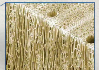
End-grain balsa at 50x magnification
